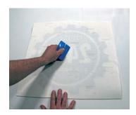
1. Place the cut vinyl sign on a clean, flat surface with the grid liner facing you. Run the squeegee over the grid liner with even pressure to secure the cut vinyl to the masking layer. SEE FIG. 1.
