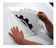
5. Once the first half is installed, remove all of the masking tape that you used to secure the material and install the second half. Remember to slowly pull away the masking layer with the graphic at a 45° angle to prevent stretching or tearing. SEE FIG. 5.
