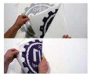
3. Choose one side and remove the corner tape. Gently and slowly pull away the masking layer with graphic at a 45° angle to prevent stretching or tearing. Stop when you reach the center tape line SEE FIG. 3A. Hold the exposed film as you use the utility knife to cut away the loose grid liner. SEE FIG. 3B.
