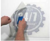
**6.** Firmly apply the remaining cut vinyl using your squeegee over the entire decal in both vertical and horizontal directions. **SEE FIG. 6.**
