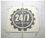
2. Using a tape measure, measure your surface area to find the center point or desired location for installation. Place the cut vinyl (grid liner down) against the desired surface, with the masking layer facing you. Place a strip of masking tape down the center and secure all four corners. SEE FIG. 2.
